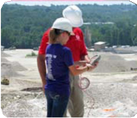
2010 Camp participant at Capital Quarry programming electronic detonator on a surface shot
